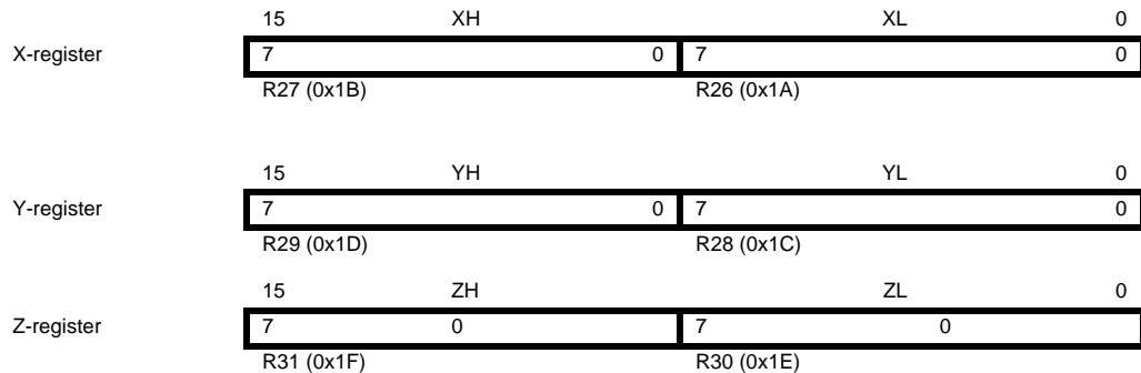
Figure 6-3. The X-, Y-, and Z-registers
